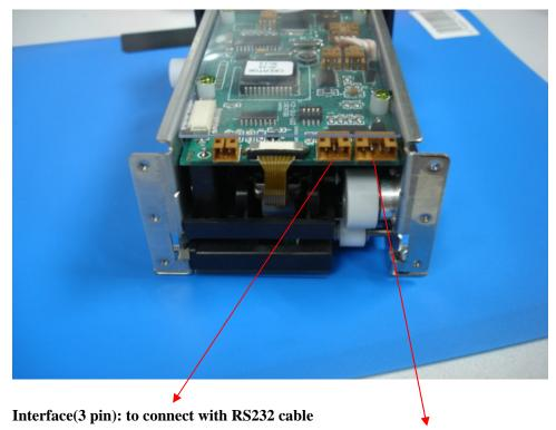
Interface(4 pin): to connect with Power cable
