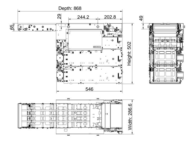
Above is the two cassettes height, with the increase of every cassette, the height shall be added by 142.5mm.
