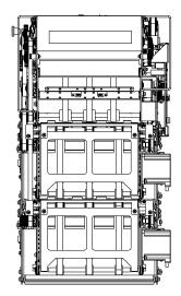
Above is the two cassettes height, with the increase of every cassette, the height shall be added by 142.5mm.
