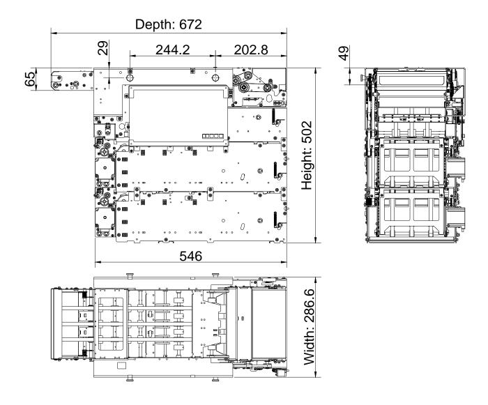
Above is the two cassettes height, with the increase of every cassette, the height shall be added by 142.5mm.
